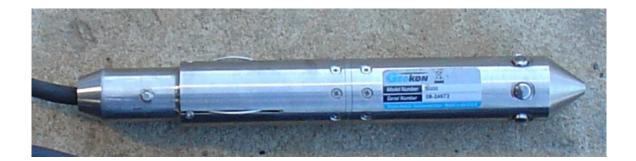
MMS initially acquired the USBM cell for use at a mine in Queensland to determine the 3D stress field, where a previous attempt at overcoring CSIRO HI Cells in the same rock unit failed. A satisfactory bond between the HI Cells and the pilot hole could not be achieved.
